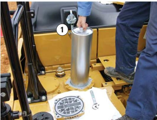
The capsule filter (1) is designed to take out impurities and help you avoid system contamination and accidental spilling. The self-contained, maintenance-friendly filter is easy to remove with a simple wrench. It can take out impurities as small as beta 10 – particles so tiny you cannot see them with the eye. A sensor lets you know if there is a clog or if pressure exceeds a certain level so you can take action.
