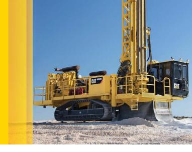
Favored by contractors, the MD6290 drills hole diameters ranging from 152-241 mm (6-9.5 in) with bit load force of up to 23 373 kg (52,321 lb). MD6290 has capability to drill depths up to 52.7 m (173 ft). The Cat® MD6290 is a diesel driven drill with top rotary head drive for both rotary and high pressure DTH drilling applications.
