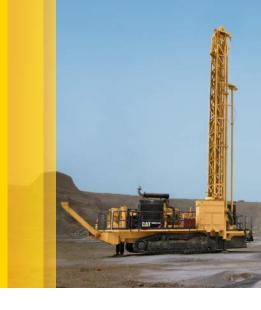
With bit load force of 24 000 kg (52,911 lb) and the capability to drill depths up to 55.47 m (182 ft) the MD6240 is well equipped to drill in hard or soft rock applications for hole size ranging from 152-244 mm (6-9.625 in). Our 15 m (49 ft) mast is ideal for single pass, high-production drilling. Many features incorporated into design of this drill assure higher productivity at lower operational cost.
