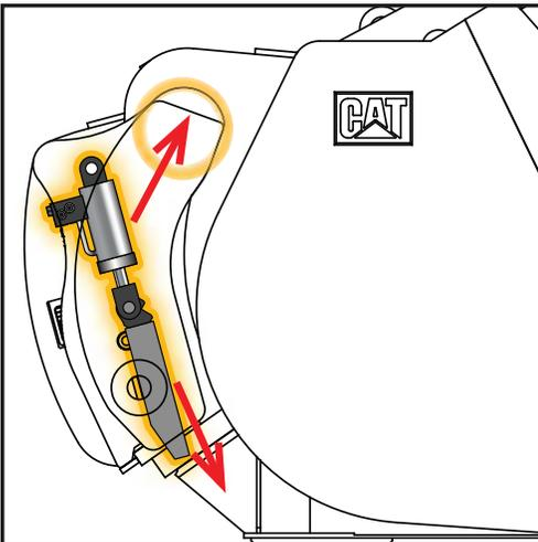
The advanced wedging mechanism of the Fusion Coupler creates a tight, rattle-free fit. This new lock up system eliminates play and wear – resulting in a long service life.
