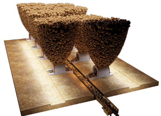
FIGURE 3: Continuous haulage system at production level
