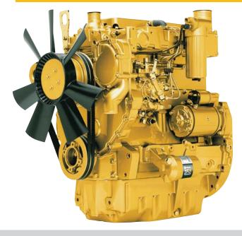
The Cat 3054C engine has been designed to meet U.S. EPA Tier 2 and EU Stage II equivalent emission standards. This engine incorporates a time-proven mechanical governor and a low-pressure fuel injection system that are major contributors to the improvement of fuel system robustness, high fuel efficiency, and ease of troubleshooting. High filtration performance from the primary filter incorporating a water separator and a secondary filter also help to improve fuel filtration system reliability.
