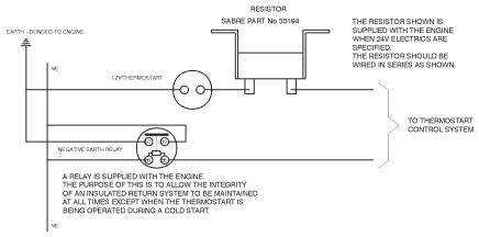
CIRCUIT DIAGRAM TO SUIT WIRING OF THERMOSTART AND EARTH RELAY FOR THE 6TWGM ENGINE.
