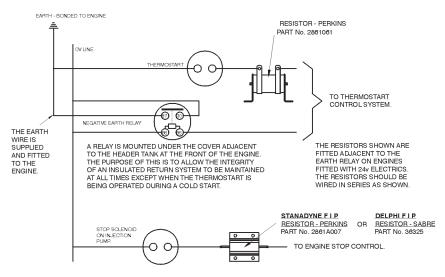
CIRCUIT DIAGRAM - EARTH RELAY AND RESISTORS FOR THE 6TG2AM ENGINE.
