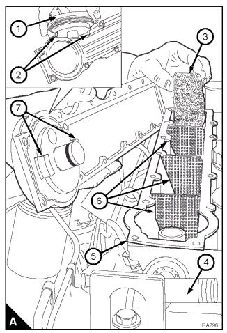
and valve assembly into position on the breather body. Loosely fit the fasteners. Tighten the fasteners gradually and evenly to 3 Nm (2.2 lbf ft) 0.3 kgf m.
