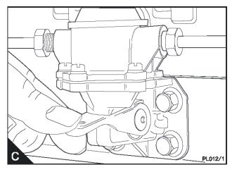
**6.** Loosen the union nuts (A1) of the high-pressure pipes at two of the atomisers.
