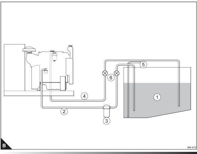
In some cases it is necessary to have a number of fuel tanks in order to achieve the required operating range. In such cases, where possible, one tank should be regarded as the main tank for each engine and the other tanks should be arranged so that they will drain into the main tank by gravity. If a gravity system is not possible, then the system shown in figure (C) should be used.
