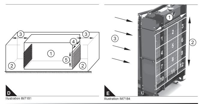
It is best to draw up a grid with each cell being of equal area. Air velocity readings are then averaged, to give a total average air velocity through the opening. This is then multiplied by the opening area to give the volumetric air flow.
