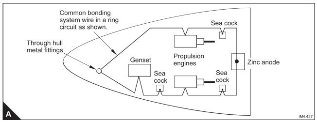
The bonding should consist of heavy stranded wire (not braiding or wire with fine strands). It is an advantage if the wire is tinned. Insulation is also an advantage and should preferably be green in colour. Although the current carried by the bonding system will not normally exceed 1 amp, the cable sizes should be generous as shown in the table below:
