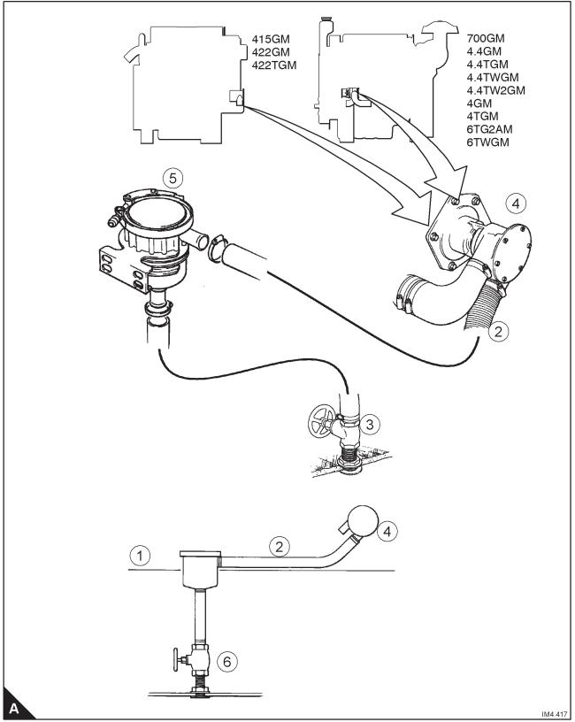
Note: Where possible mount the strainer so that the top is just above the waterline to facilitate cleaning.
