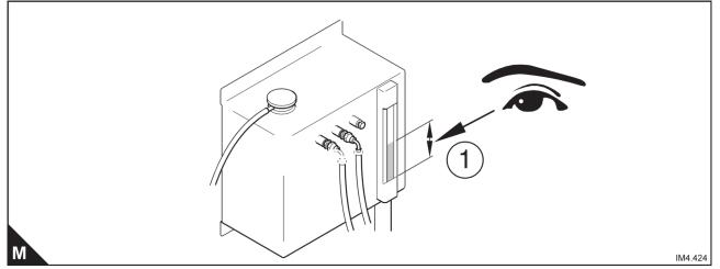
*Warning!* Hot coolant is under pressure and can cause severe burns when removing the pressure cap. First release the pressure in the system by loosening the pressure cap.
