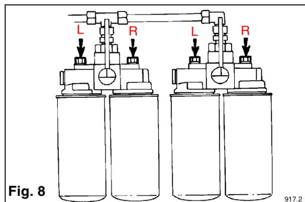
**PRIMING AND VENTING THE FUEL SYSTEM AS FITTED ON LATER 12 & 16 CYLINDER ENGINES**
