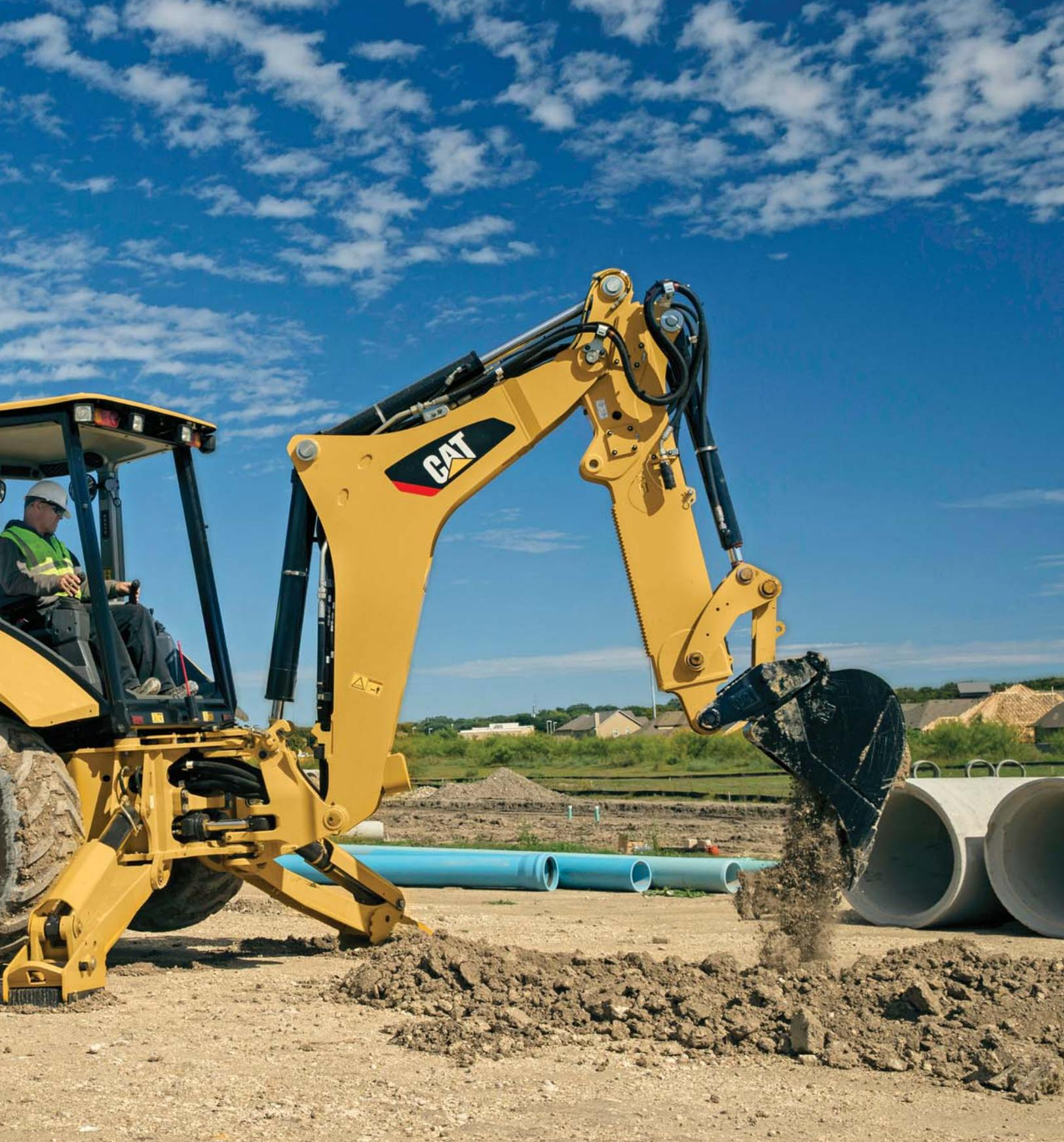
**Experience the Backhoe Loader designed around customer feedback. The Cat 420F2 Backhoe Loader puts all the machine controls at the operator's fingertips. Operate all auxiliary controls with thumb rollers. Move from job site to job site quickly and smoothly with the additional 6th gear on the autoshift transmission and optional lock-up torque converter.**
