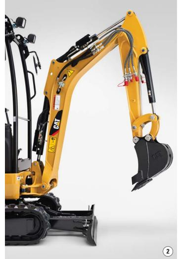
The 'ready to work' quick disconnect connections are equipped with an accumulator as standard to help make releasing and changing of tools a quick and easy task. Located close to the work tool, they reduce hose lengths and minimize potential damage.
