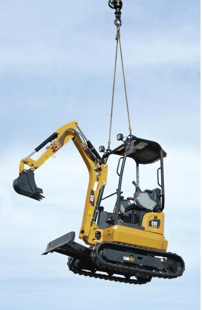
Sturdy hoisting points on the canopy roof enable the easy, safe and rapid relocation of the machine between sites or for loading of the machine onto a trailer.
