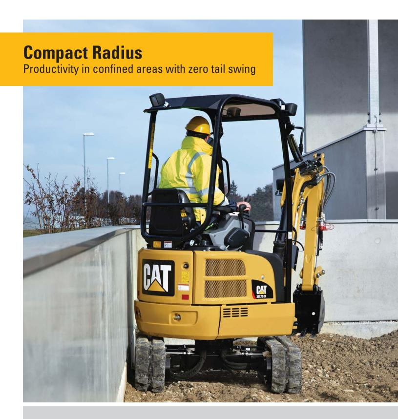
The zero tail swing Cat 301.7D CR can work comfortably in confined work areas with the machine upper frame able to slew within its track width. This compact radius design also allows you to concentrate on the work being performed without having to worry about damage to the back of the machine or site.
