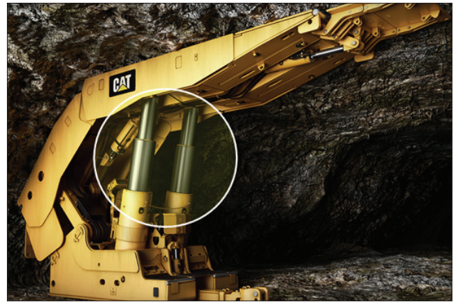
Cat ® roof support with NiL35 coated hydraulic cylinders
