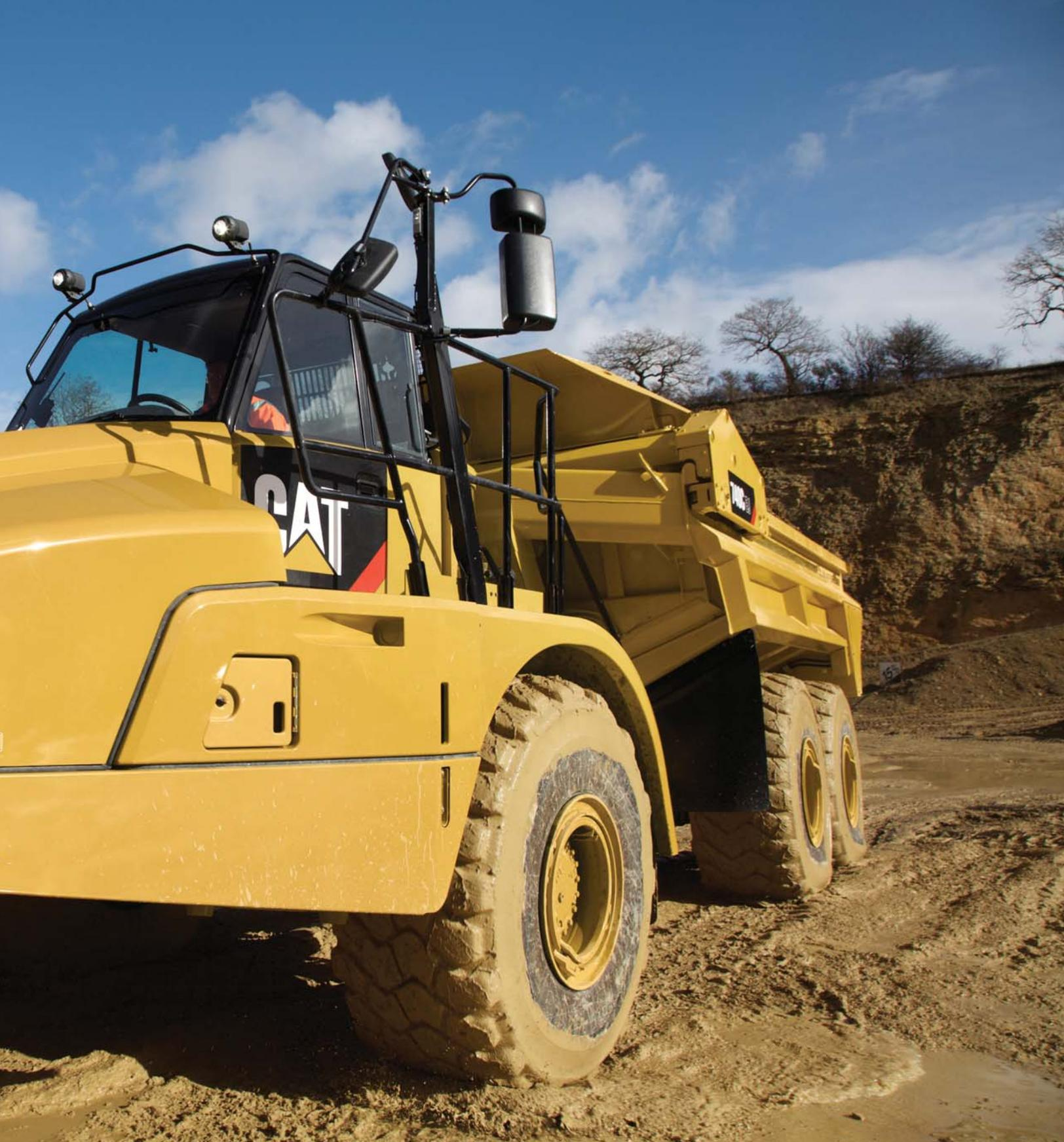
**The Cat 740C EJ with a 23 m<sup>3</sup> (30.1 yd<sup>3</sup>) 38 tonnes (42 ton) capacity offers proven reliability, durability, high productivity, superior operator comfort and lower operating costs.**
