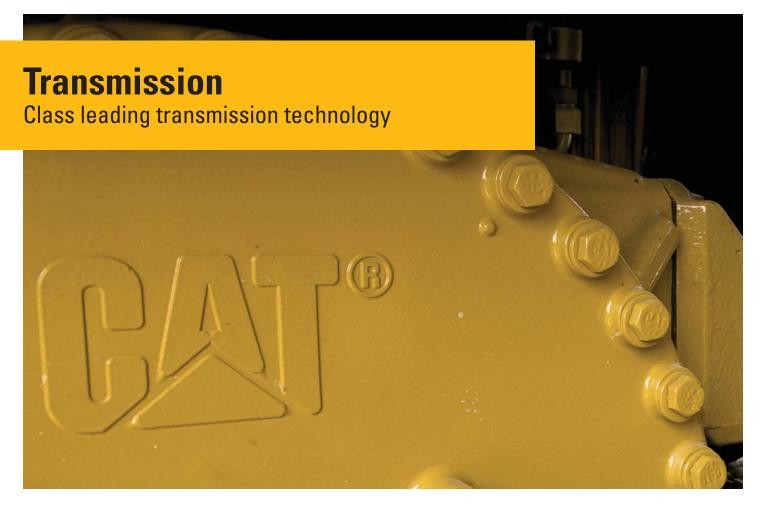
The new Cat High Density Power Shift (HDPS) nine-speed forward two-speed reverse transmission features Advanced Productivity Electronic Control Strategy (APECS) and Electronic Clutch Pressure Control (ECPC) which deliver smooth gear changes with improved acceleration and higher productivity.
