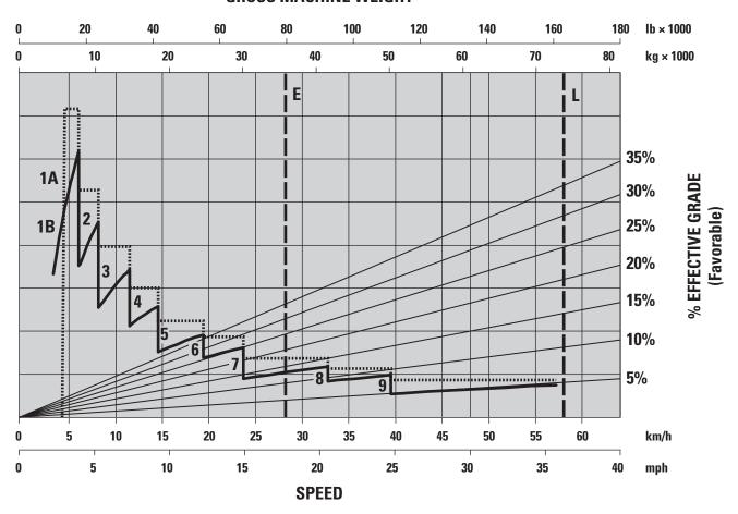
1A – 1st Gear (Converter Drive)
