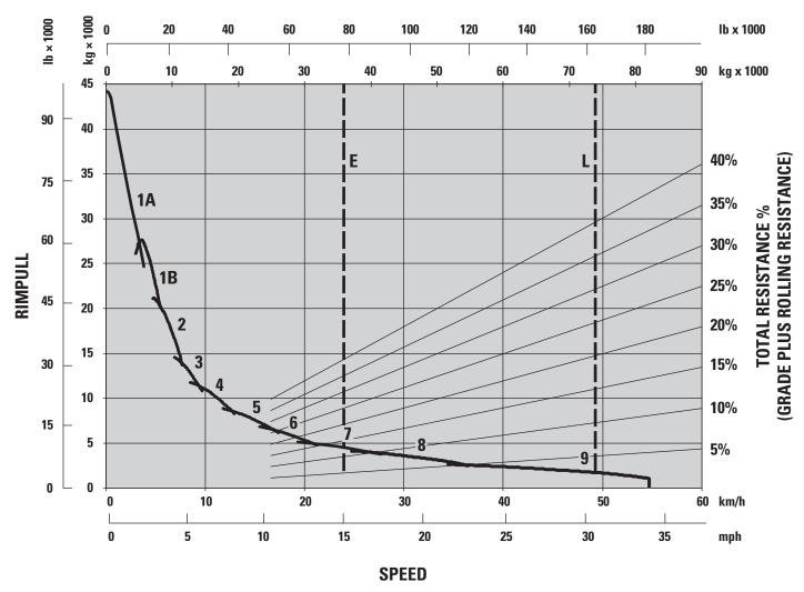
1A – 1st Gear (Converter Drive)
