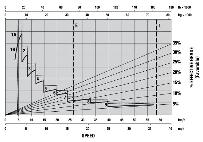
1A – 1st Gear (Converter Drive)
