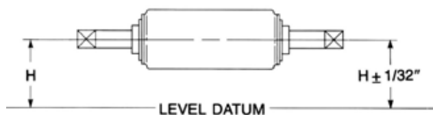
Figure TG.5 Shaft elevation settings
