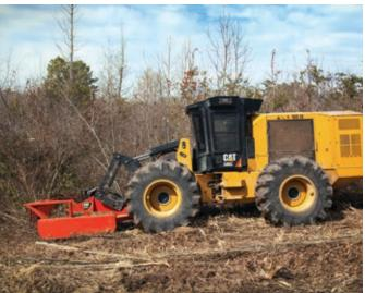
Unique operating modes, combined with complete electrohydraulic controls, provide the operator with a smoother machine with increased productivity. These modes include Creep Mode to easily adjust machine speed to improve mulching, Terrain Selection Mode to optimize performance on hills or flat ground, and Road Steer Mode for high-speed transport of the machine.
