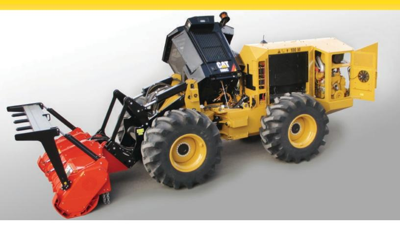
Daily service points are in easy reach on the 586C. Add hydraulic oil with the electric pump and refuel with your boots on solid ground. The tilting cab and hinged panels give you access to even more.
