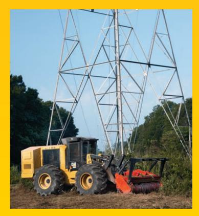
The Cat 586C Site Prep Tractor is a multi-purpose, heavy-duty machine with the muscle to run power-hungry mulchers and brushcutters. Tackle a variety of land management projects with one machine and lower your owning and operating costs. Applications include residential/commercial development, utility and pipeline right-of-way construction and maintenance, wetlands and wildlife habitat management, plantation reclamation and management, and clearing for flood control and firebreaks.
