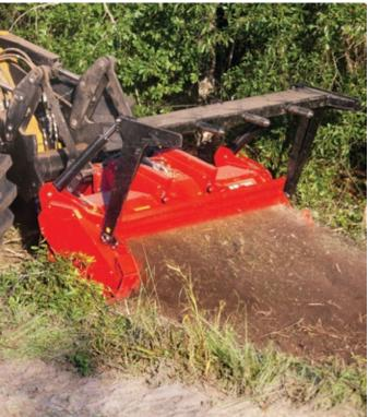
New Cat work tools have been developed to match the powerful capability of the 586C Site Prep Tractor. The Cat HM825 Mulcher and the Cat BR624 Brushcutter are available from the factory and supported by your Cat dealer. Other key 586C attachments include an attachment quick coupler and retrieval assist winch to increase versatility.
