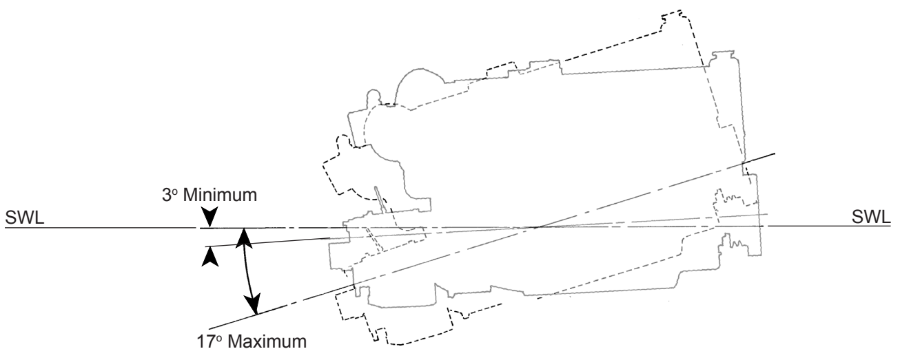
Figure 3 - When in standard form all engine models may be installed 'flywheel down' from a minimum of 3° to a maximum of 17°.
