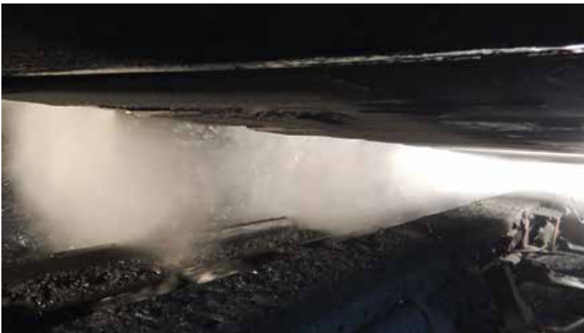
Plow system with dust suppression system ("water curtain")
