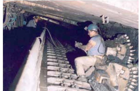
Maintenance in the plow face
