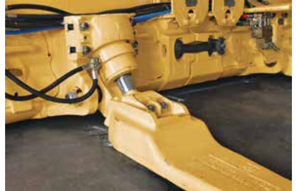
Outrigger steering cylinder for horizon control
