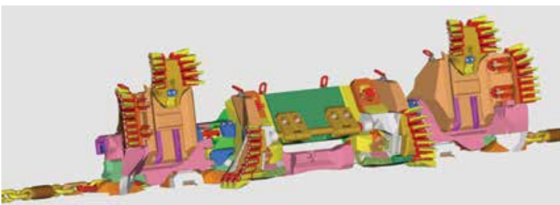
FIGURE 4. The type 2.7 triple plow body used at the U.S. Steel Mine since 1999
