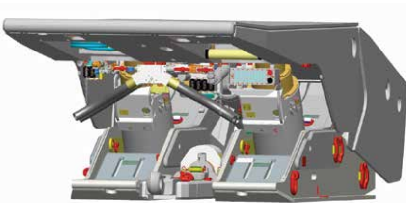
FIGURE 8. A face roof support for the newest Pinnacle plow system
