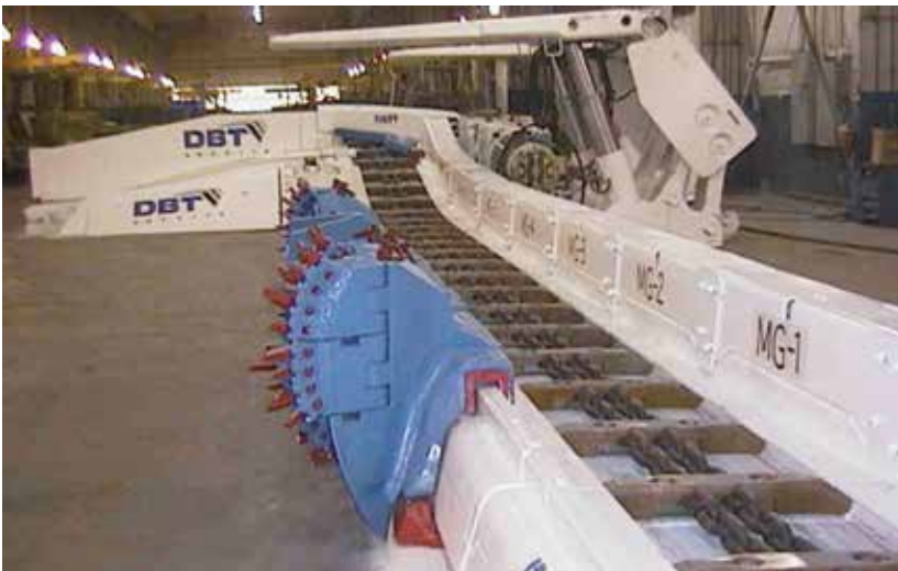
FIGURE 3. Plow system delivered for U.S. Steel #50 mine in 1999
