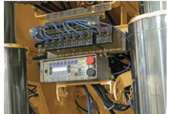
Cat PMC®-R electrohydraulic shield control system
