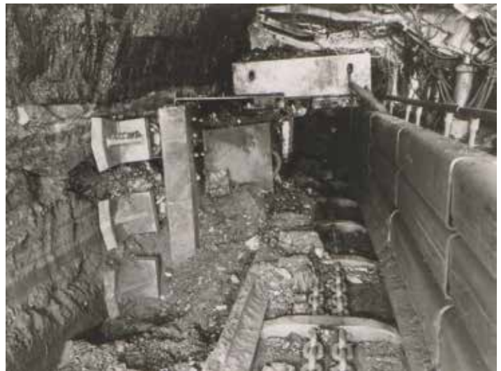
Schlagkopfhobel of Bergbau-Forschung GmbH (activated through hydraulic pick hammers on both sides of the machine, which was pulled by a plow chain)
