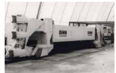
Activated plow from the GHH company (high-pressure water jets pre-cut the coal behind the mechanical bits)
