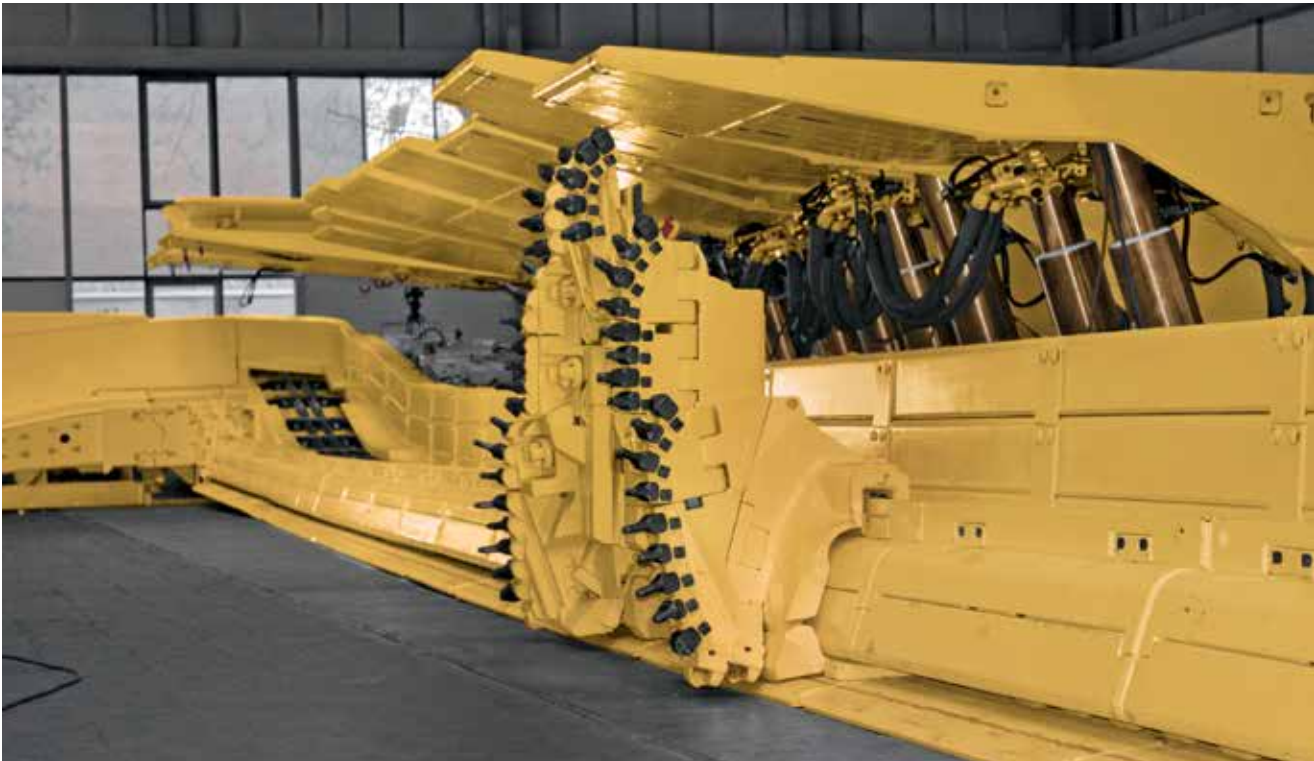
Surface compatibility test for the Cleveland Cliffs plow system in 2010 in the USA
