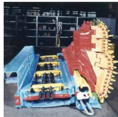
Standard plow systems at DBT Deutsche Bergbau-Technik in 1995: Reissshakenhobel® S 4N (above) and Gleithobel® 9-38 ve 5.7 (below)
