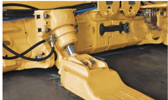
Horizon control for easy height adjustments
