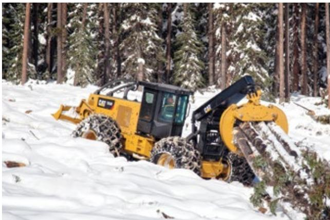
The new hydraulic system gives the D Series more speed, increased multifunctioning capability and greater lift capacity. This efficient load sense system with variable displacement pump continually monitors hydraulic power requirements and provides power based on demand to save fuel.
