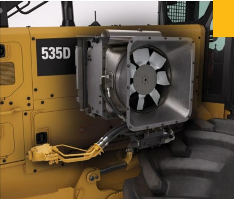
The high capacity cooling system and on-demand hydraulically driven reversing fan keep the machine running at the proper operating temperature, optimizing performance, durability and fuel efficiency. The system, designed to meet the cooling requirements of the 555D, is common to all models, boosting fuel efficiency and capacity in the smaller models.
