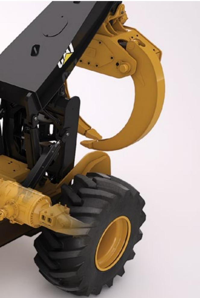
Power to the ground is an advantage of the Cat D Series. The axles are designed specifically for the skidder application and the gear ratios cause the power to be generated in the axles reducing torque in the transmission and drivelines extending their life. Both drawbar performance and durability are improved.
