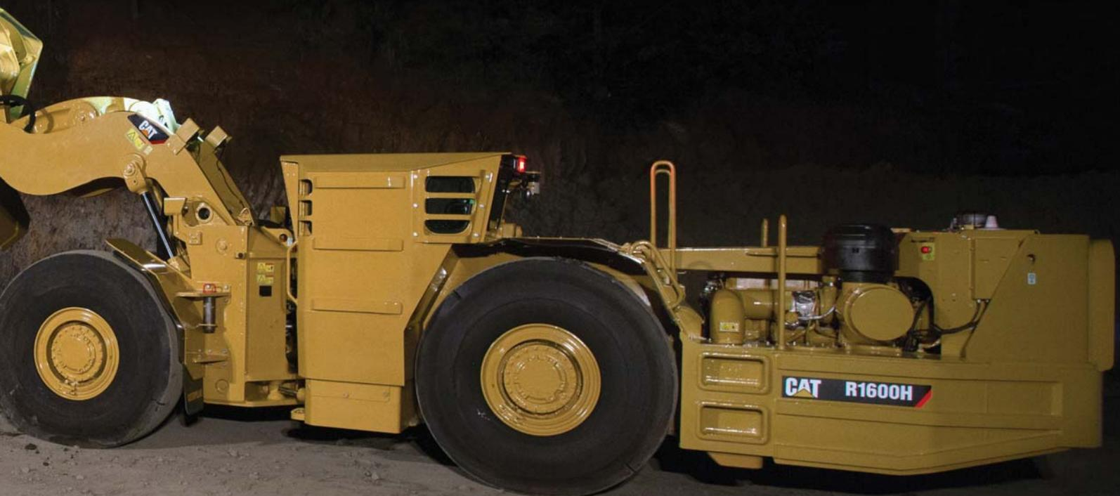
**The R1600H underground loader is well matched to the AD30 underground truck for a loader and truck combination. The R1600H can easily load the AD30 truck fitted with a dump body or ejector body configuration using a standard dump bucket or if restricted by height the ejector bucket option could be used on the loader.**
