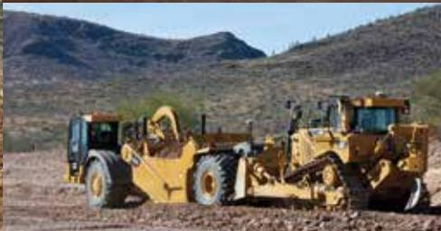
Versatile Cat dozers keep mine sites operating at peak productivity and are essential machines for dozens of jobs, such as truck dump and site maintenance, leveling the bench after blasting, establishing a general gradient and width for the bench, and working alongside loaders, shovels and draglines to support the performance of the loading and hauling fleet.
