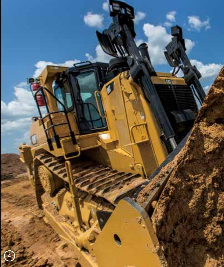
3. Automatic Ripper Control monitors the dozer speed with the ROPS mounted GNSS to automatically adjust engine speed and ripper depth to minimize track slip. This feature reduces operator fatigue and decreases wear and tear on the machine.
