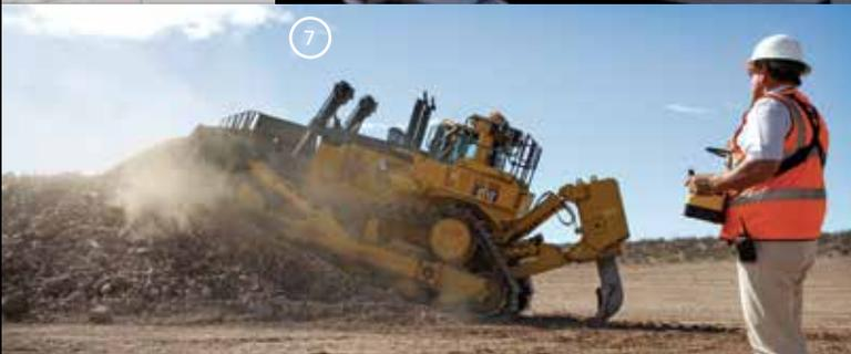
7. Command for dozing allows the operator to control the machine using a lightweight over-the-shoulder console. The system keeps operators out of potentially harmful environments and limits exposure to vibration, dust and noise. The operator console can be used for line-of-sight control up to 400 meters (1,312 feet).
