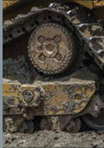
Cat dozers have an elevated sprocket and fully suspended undercarriage, which work together to provide increased traction and a smoother ride in addition to improved production and longer component life.
