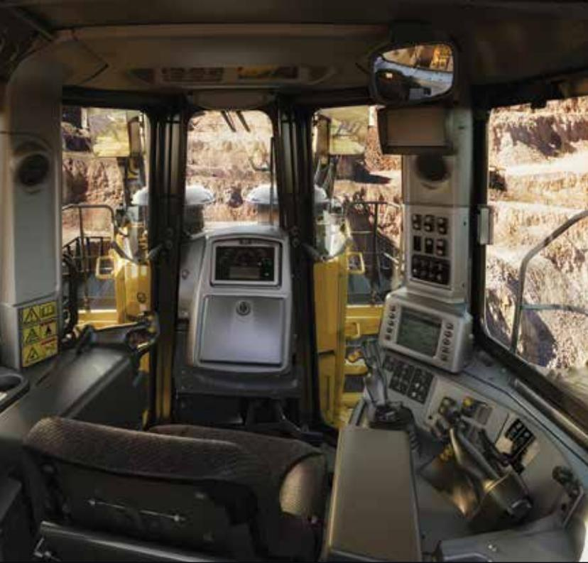
The Cat T Series cab is designed for operator comfort, safety and productivity, with ergonomic controls that reduce fatigue, enhanced visibility, and intuitive monitoring systems and information displays. Features include a fully adjustable air suspension seat, reduced sound levels and an automatic climate control system.
