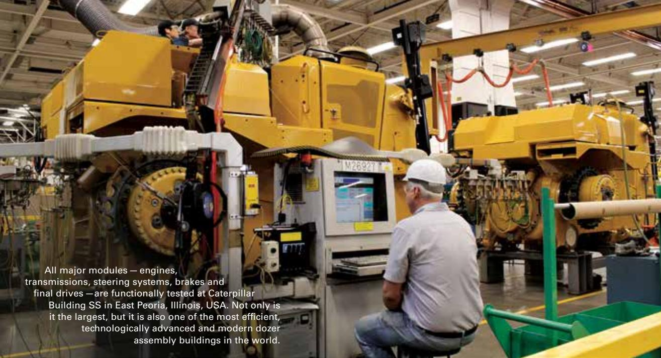
All major modules — engines, transmissions, steering systems, brakes and final drives — are functionally tested at Caterpillar Building SS in East Peoria, Illinois, USA. Not only is it the largest, but it is also one of the most efficient, technologically advanced and modern dozer assembly buildings in the world.
