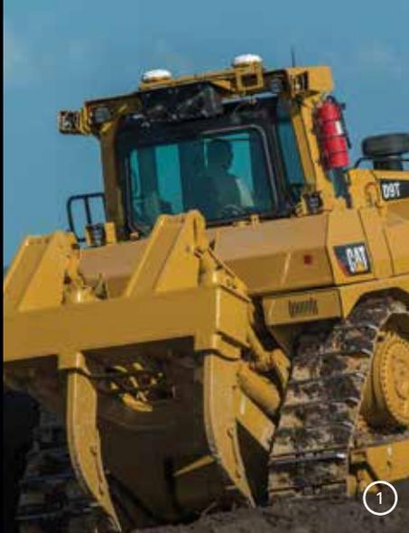
1. Cat Grade Control 3D uses dual ROPS mounted GNSS antennas and in-cylinder position sensors to provide precise positioning of the cutting edge, eliminating the need for masts and cables on the blade. The system also reduces the need for grade staking and grade checking; as a result, fewer people are required on the job site, which lowers personnel costs and enhances safety.
