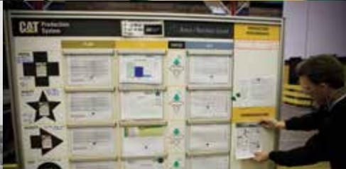
The innovative Caterpillar Production System is helping to transform our manufacturing systems and set new standards for quality, safety and speed in the industry. The scoreboard above is used to track daily metrics at the factory, section, and area levels to provide visual status updates.
