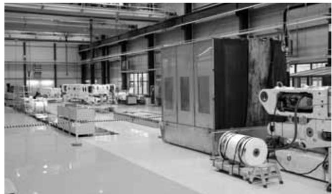
*Three shearers at different stages in the manufacturing process: From the shearer on the left which is ready for equipping to the one on the right which has successfully completed all test procedures and is being prepared for shipping.*
