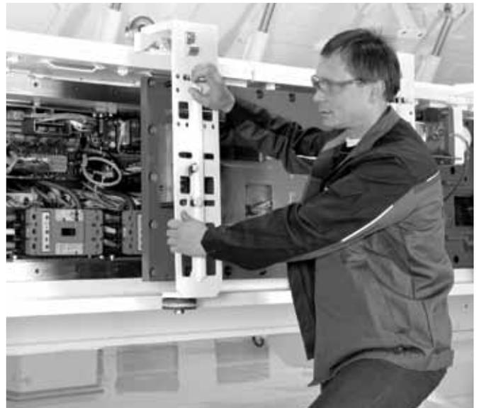
*The robust mainframe protects the electrical boxes from cutting and haulage forces; door handling system for easy access to the electrical compartments.*
