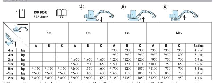
Lifting capacities were calculated with a machine equipped with a 0.22 m³ capacity standard bucket. The difference between the weight of a work tool attachment and the standard bucket must be subtracted.
