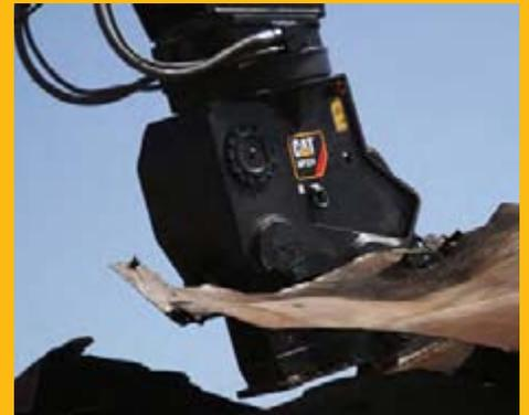
**Tank Shear (TS) Jaw**
