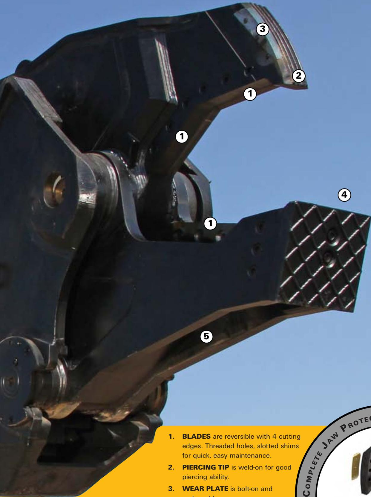
1. **BLADES** are reversible with 4 cutting edges. Threaded holes, slotted shims for quick, easy maintenance.
