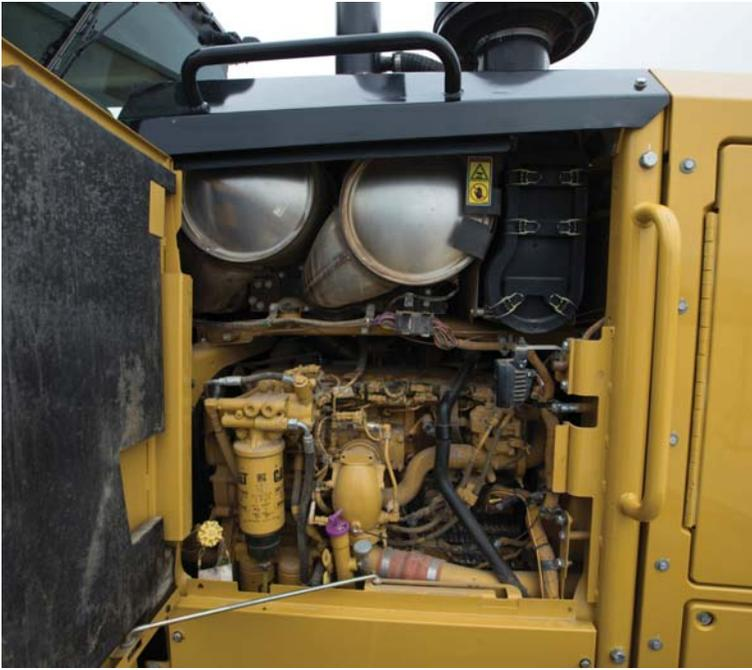
Emissions reduction technology on the M Series 3 Motor Grader is designed to be transparent, with no action required from the operator. There is no need to stop. Regeneration runs automatically at cold start-up and, if needed, in the background while you work.
