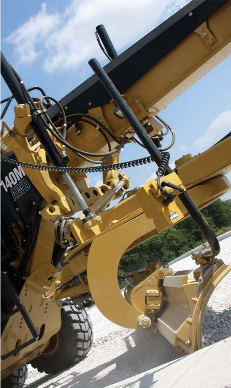
Caterpillar designs motor grader frame and drawbar components to give you performance and durability. The one-piece forged steel circle stands up to high stress loads, and a sacrificial wear system helps keep your service time and costs down.
