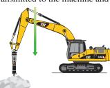
**Hammer Work.** The front parts automatically follow the hammer while penetrating the rock. Blank shots or excessive force on the hammer are avoided resulting in longer life for the hammer and the machine. Similar advantages with vibratory plates.
