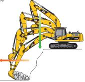
**Truck Loading.** Loading trucks from a bench is more productive and fuel efficient as the return cycle is reduced while the boom down function does not require pump flow.
