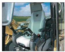
**Consoles.** Redesigned consoles feature a simple, functional design to reduce operator fatigue, ease of switch operation and excellent visibility. Both consoles have attached armrests with height adjustments.
