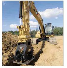
**Tracks.** The 324D comes standard with grease lubricated tracks. The track links are assembled and sealed with grease to decrease internal bushing wear, reduce travel noise and extend service life lowering operating costs.
