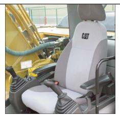
**Seat.** The air suspension seat is standard in the 328D LCR, provides a variety of adjustments to suit the operator'size and weight including fore/aft, height and weight. Wide adjustable armrest and a retractable seat belt are also included
