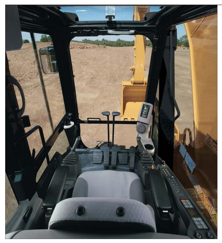
**Operator Station.** The workstation is spacious, quiet and comfortable, assuring high productivity during a long workday. The attachment switches, key switch and throttle dial are conveniently located on the right-hand wall. The monitor is easy to see and maximizes visibility. The ROPS Cab air filter is accessible at ground level.
