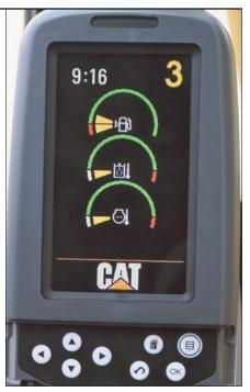
**Monitor.** The monitor is a full color 400 x 234 pixels Liquid Crystal Display (LCD) graphic display. The angle can be adjusted to minimize sun glare and has the capability of displaying information in twenty-seven different languages.
