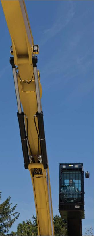
You know that a material handler works only as good as its front linkage is able to handle the job. The MH3059's boom and stick are purpose built for the loads encountered in bulk material handling applications, able to withstand extreme loading conditions.
