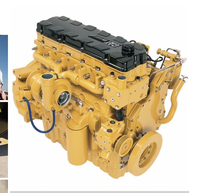
More power when you need it, the Cat C9 ACERT large displacement engine optimizes machine performance and enhances fuel efficiency while meeting Tier 3/Stage IIIA emission regulations. The C9 is an 8.8 L (537 in³), in-line 6 cylinder engine rated at 242 kW (325 hp). This market proven Cat engine produces enough power to run simultaneous machine operations.
