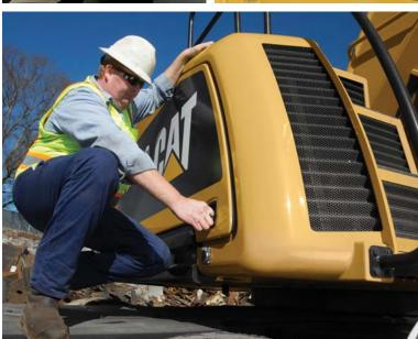
To ease serviceability on the MH3059, all primary service points are conveniently located under a single access service panel on the right side of the machine or beneath the top engine access panel. Easily locate components with the engine and cooling system's longitudinal layout. Both panels are hinged with gas struts, ensuring that one technician can easily access all maintenance points.
