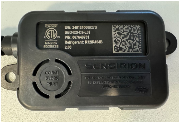
FIGURE 6. Example of Clear, Unobstructed Sensor Inlet
