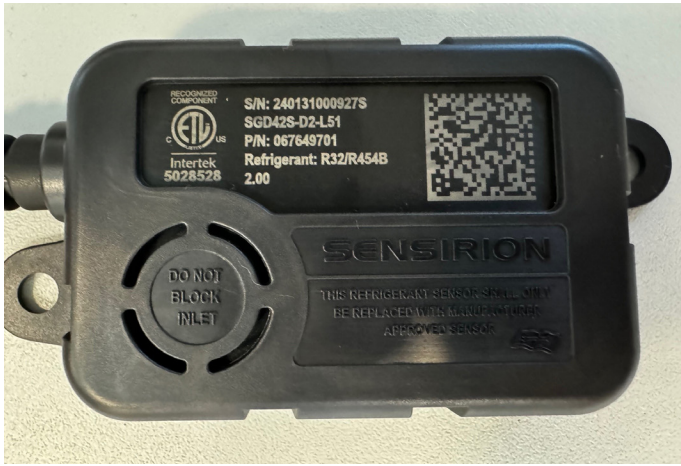
FIGURE 8. Example of Clear, Unobstructed Sensor Inlet
