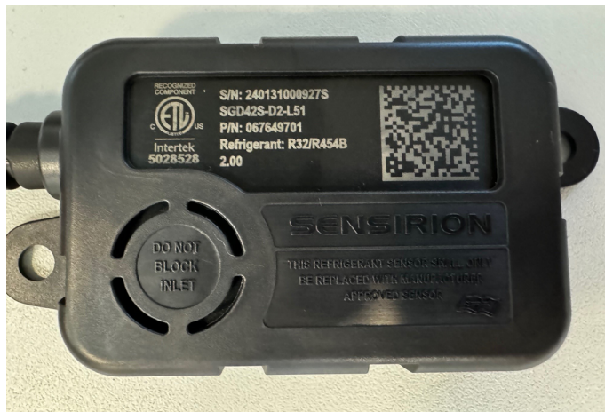
FIGURE 7. Example of Clear, Unobstructed Sensor Inlet
