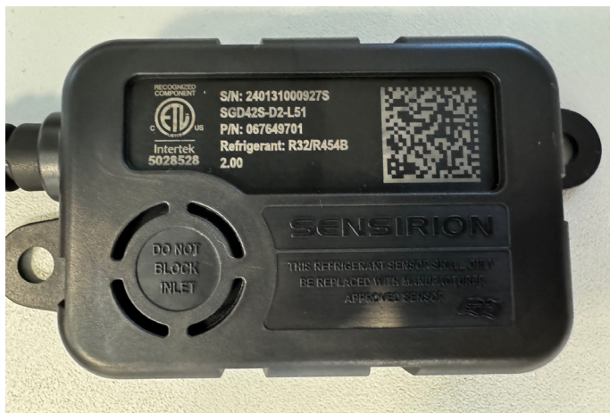
FIGURE 6. Example of Clear, Unobstructed Sensor Inlet
