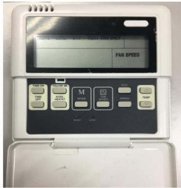
Permanent Memory - Maintains clock, fan speed and mode of operation settings following power outages.
