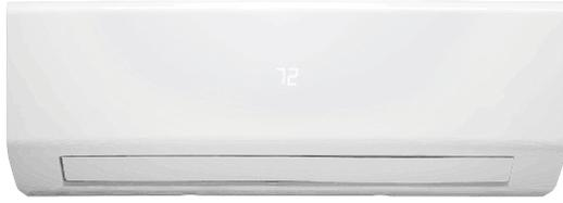
Low-sound, three-speed Wall Mount with LED display offers three access points for refrigerant outlet pipes: left, right or rear. The front panel can be raised for accessible wiring and maintenance. Swing louver angles to 90°. Unit installs horizontally on a vertical wall.
