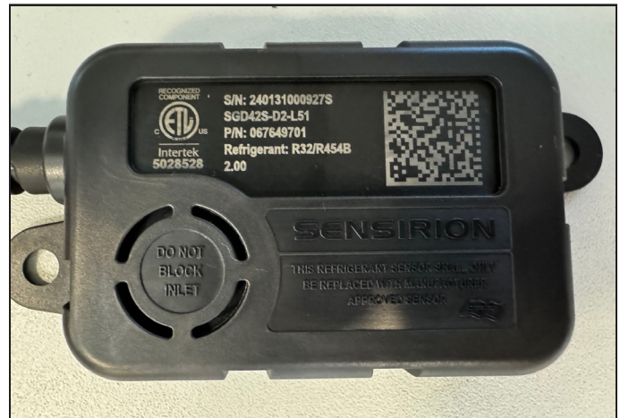
FIGURE 14. Example of Clear, Unobstructed Sensor Inlet
