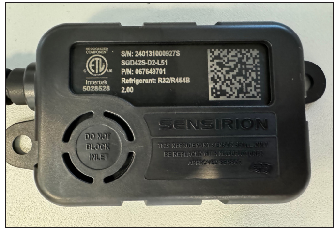
FIGURE 10. Example of Clear, Unobstructed Sensor Inlet
