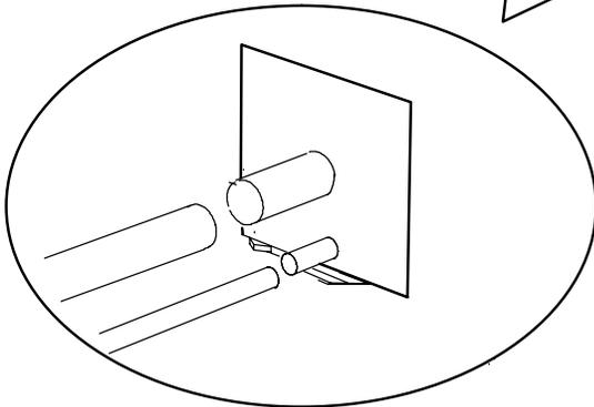
**G** PLACE A WET RAG AGAINST PIPING PLATE AND AROUND THE SUCTION LINE CONNECTION.
