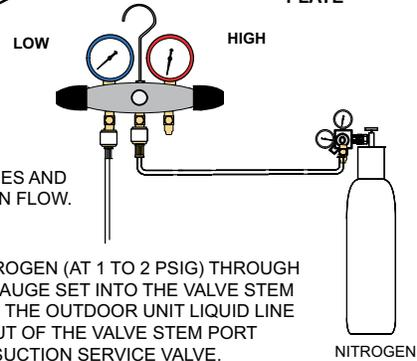
FLOW REGULATED NITROGEN (AT 1 TO 2 PSIG) THROUGH THE REFRIGERATION GAUGE SET INTO THE VALVE STEM PORT CONNECTION ON THE OUTDOOR UNIT LIQUID LINE SERVICE VALVE AND OUT OF THE VALVE STEM PORT CONNECTION ON THE SUCTION SERVICE VALVE.
