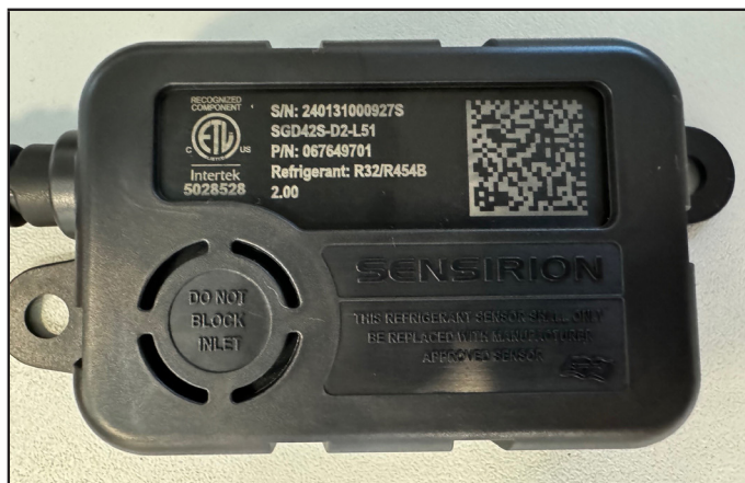
FIGURE 2. Example of Clear, Unobstructed Sensor Inlet
