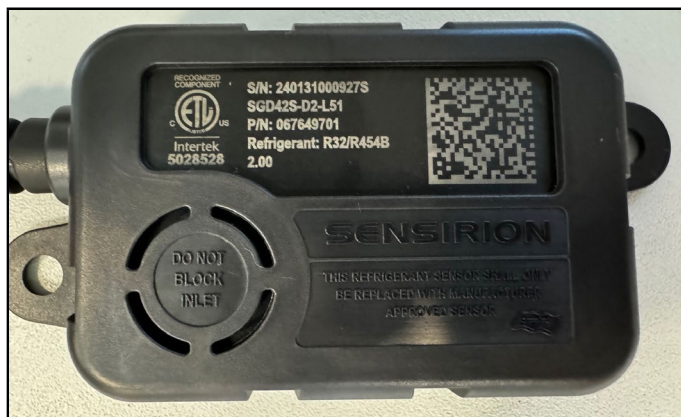
FIGURE 22. Example of Clear, Unobstructed Sensor Inlet
