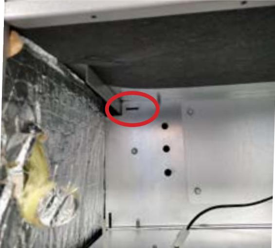
Figure 5. Notch for Control Panel Relocation
