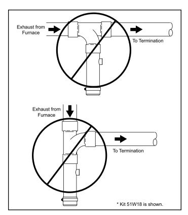
Figure 50. Crawl Space Vent Pipe Drain Trap
