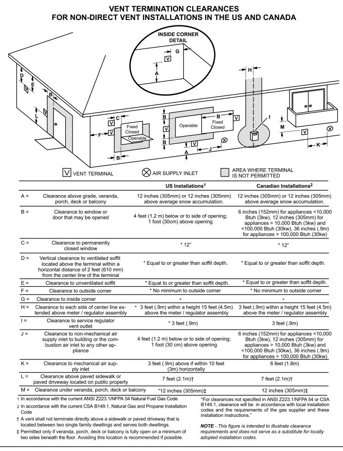
Figure 34. Vent Termination Clearances for Non-Direct Vent Installations
