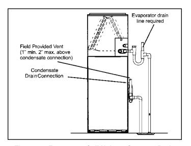
Figure 55. Evaporator Coil Using a Separate Drain
