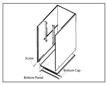
Figure 16. Removing the Bottom Panel
