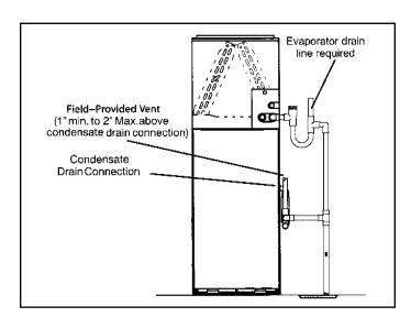
Figure 56. Evaporator Coil Using a Common Drain
