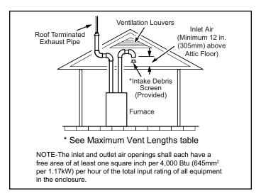
Figure 10. Equipment in Confined Space (Inlet Air from Ventilated Attic & Outlet Air to Outside)
