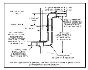
Figure 47. Non-Direct Vent Field Supplied Wall Termination Extermination
