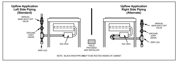
Figure 61. Gas Piping Upflow Applications
