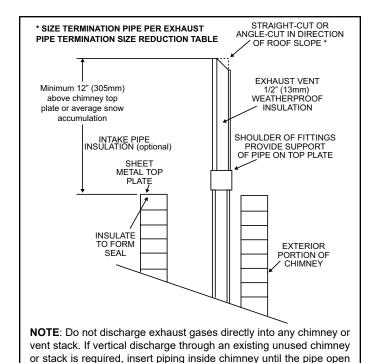
Figure 48. Non-Direct Vent Application Using Existing Chimney
