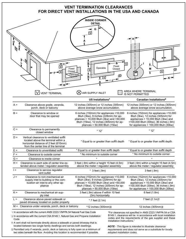
Figure 35. Vent Termination Clearances for Direct Vent Installations
