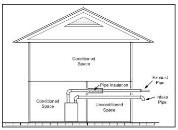
Figure 33. Insulating Exhaust Pipe in an Unconditioned Space
