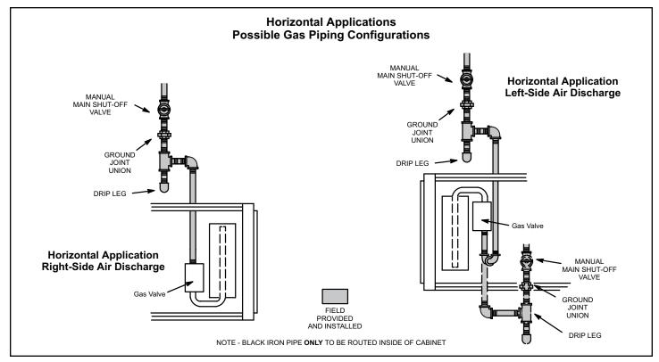
Figure 62. Gas Piping Horizontal Applications
