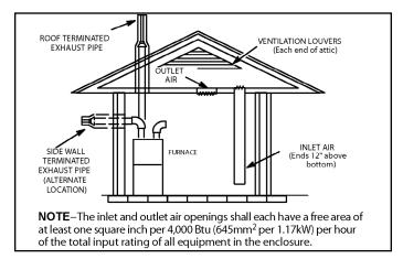
Figure 7. Equipment in Confined Space - All Air from Outside
