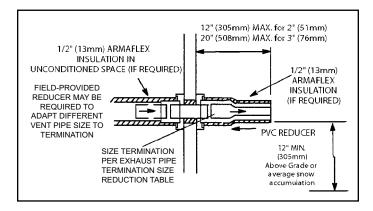
Figure 46. Non-Direct Vent Field Supplied Wall Termination
