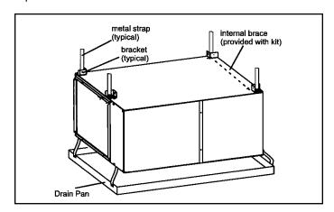
Figure 19. Typical Horizontal Application
