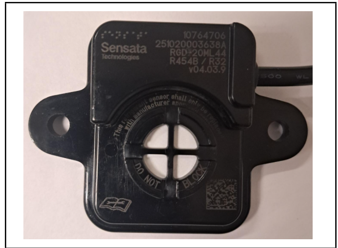
Figure 30. Example of Clear, Unobstructed Sensor Inlet
