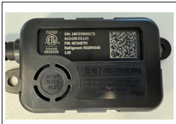
Figure 29. Example of Clear, Unobstructed Sensor Inlet
