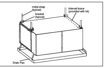
Figure 19. Typical Horizontal Application
