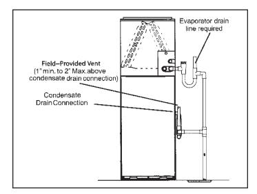
Figure 56. Evaporator Coil Using a Common Drain
