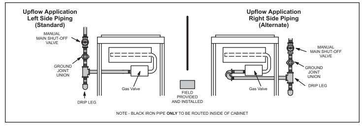
Figure 61. Gas Piping Upflow Applications
