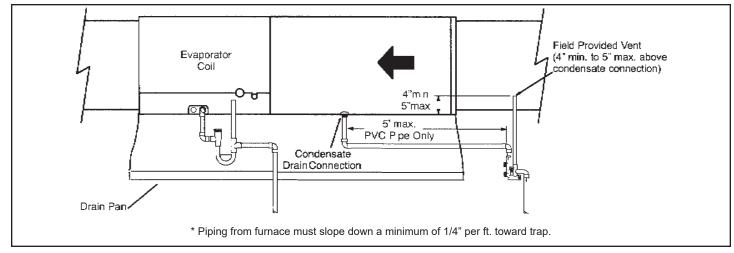
Figure 54. Evaporator Coil Using a Separate Drain (Unit shown in horizontal right-hand discharge position)
