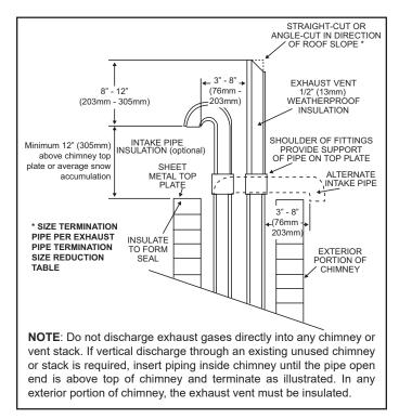
Figure 43. Direct Vent Application Using Existing Chimney
