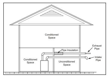
Figure 33. Insulating Exhaust Pipe in an Unconditioned Space
