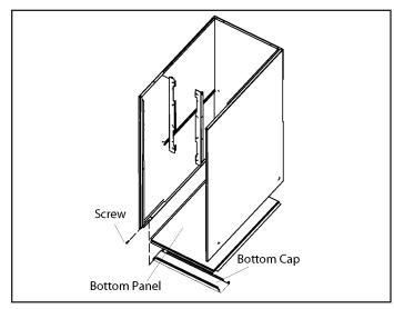
Figure 16. Removing the Bottom Panel
