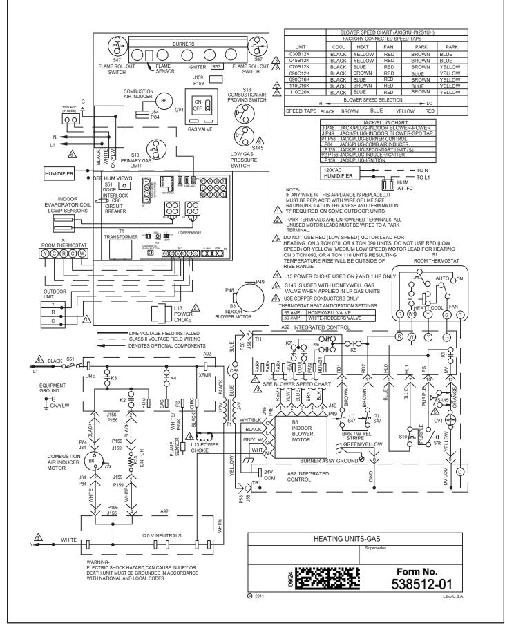
Figure 66. Typical Wiring Diagram
