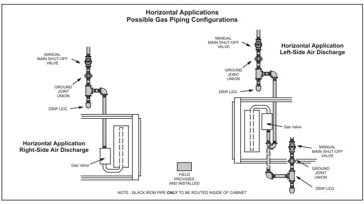
Figure 62. Gas Piping Horizontal Applications Gas Pipe Capacity - FT<sup>3</sup>/HR (kL/HR)
