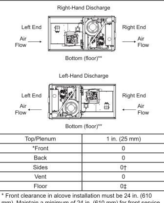
\* Front clearance in alcove installation must be 24 in. (610 mm). Maintain a minimum of 24 in. (610 mm) for front service access.
