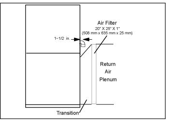
Figure 14. Side Return Air (with Transition and Filter)
