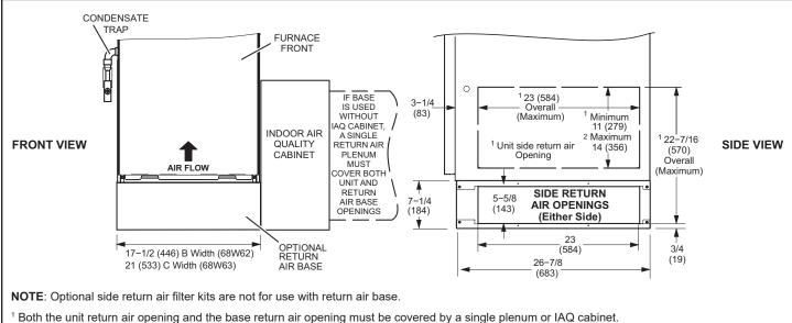
Minimum unit side return air opening dimensions for units requiring 1800 cfm of air and over (W x H): 23 x 11 in. (584 x279 mm).
