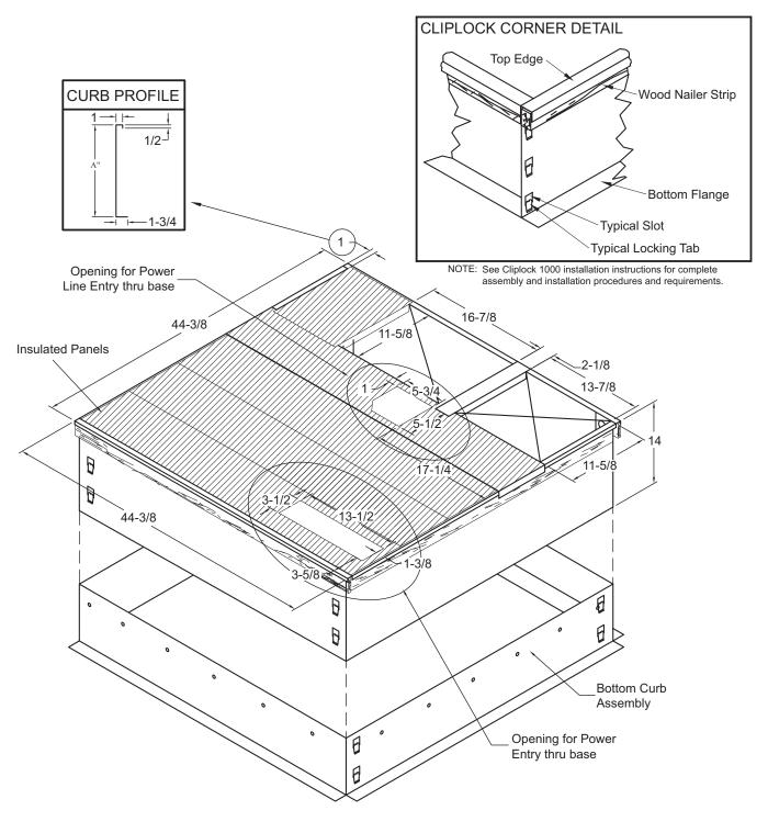
NOTE - If bottom entry is used, condensate from the heat exchanger may leak during warm ambient temperatures in humid climates. Ensure that bottom entry is watertight, if used.
