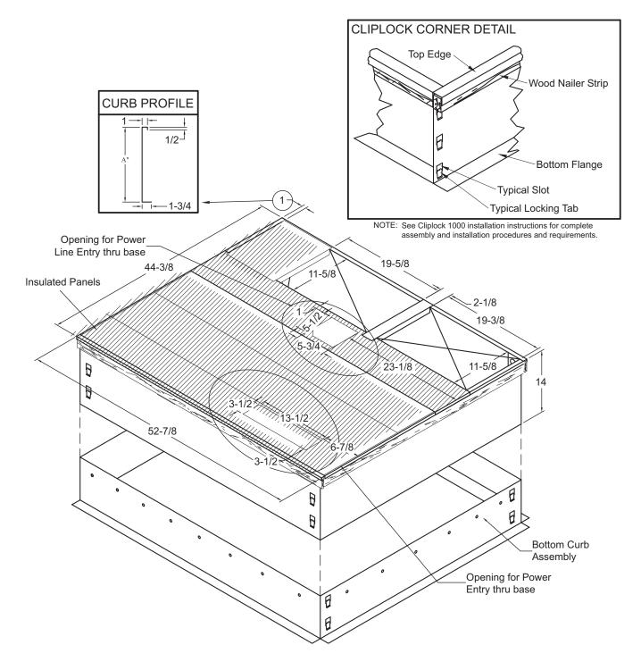
NOTE - If bottom entry is used, condensate from the heat exchanger may leak during warm ambient temperatures in humid climates. Ensure that bottom entry is watertight, if used.
