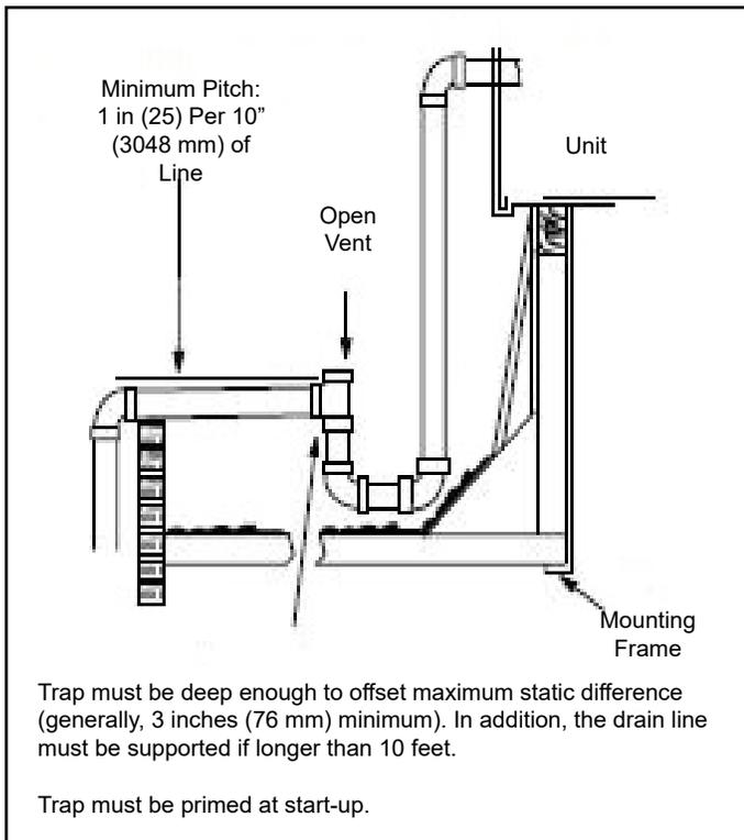
**Figure 4. Typical Condensate Drain Connection**
