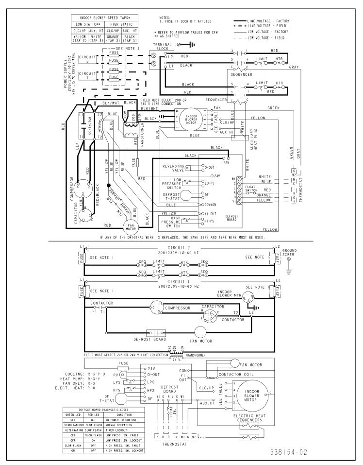
Figure 16. Wiring Diagram - MHP with Dual Circuit (3 Ton)
