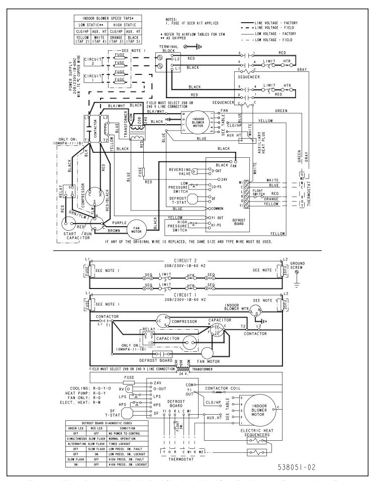
Figure 14. Wiring Diagram - MHP with Dual Circuit and Hard Start Enabled (0.75 Ton through 2.5 Ton) of 18 Issue 2240 50
