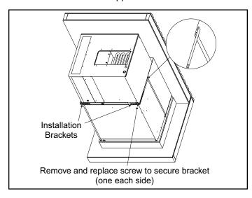
Figure 5. Securing Unit
