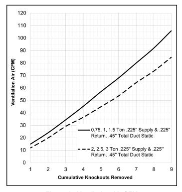
Figure 9. Ventilation Air CFM
