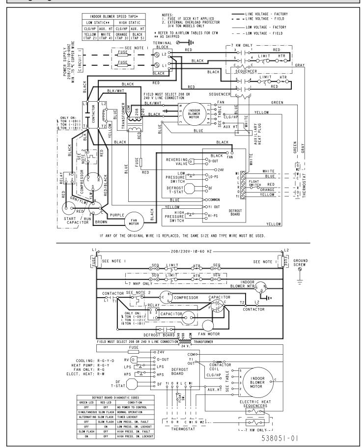
Figure 13. Wiring Diagram - MHP with Single Circuit and Hard Start Enabled (0.75 Ton through 2.5 Ton)
