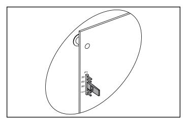
Figure 11. Defrost Interval Timing Jumper
