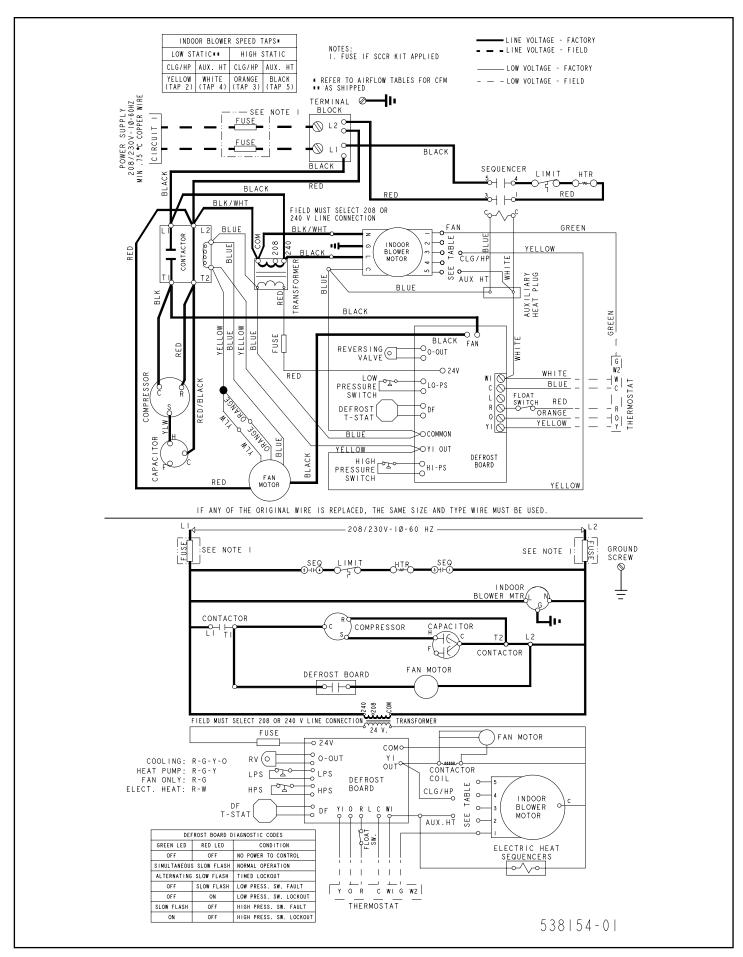
Figure 15. Wiring Diagram - MHP with Single Circuit (3 Ton)
