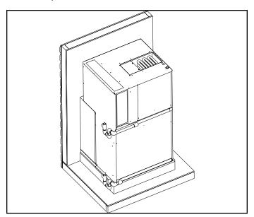
Figure 7. Condensate Drain Installation
