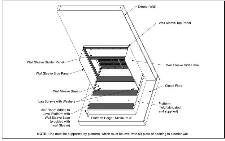
Figure 3. Wall Sleeve and Louver Kit Installation
