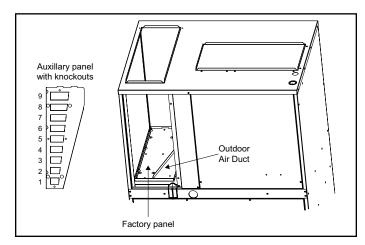
Figure 8. Auxiliary and Factory Panel for Ventilation Air
