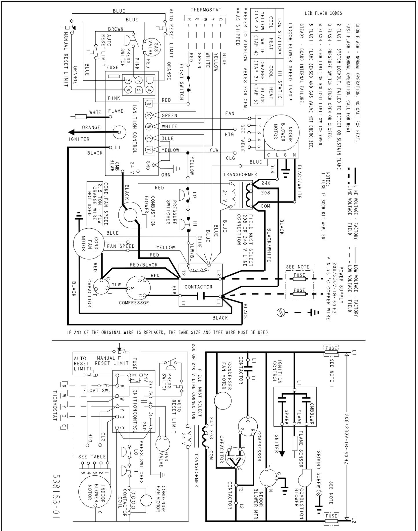
Figure 13. Wiring Diagram - MGE 2.5 Ton
