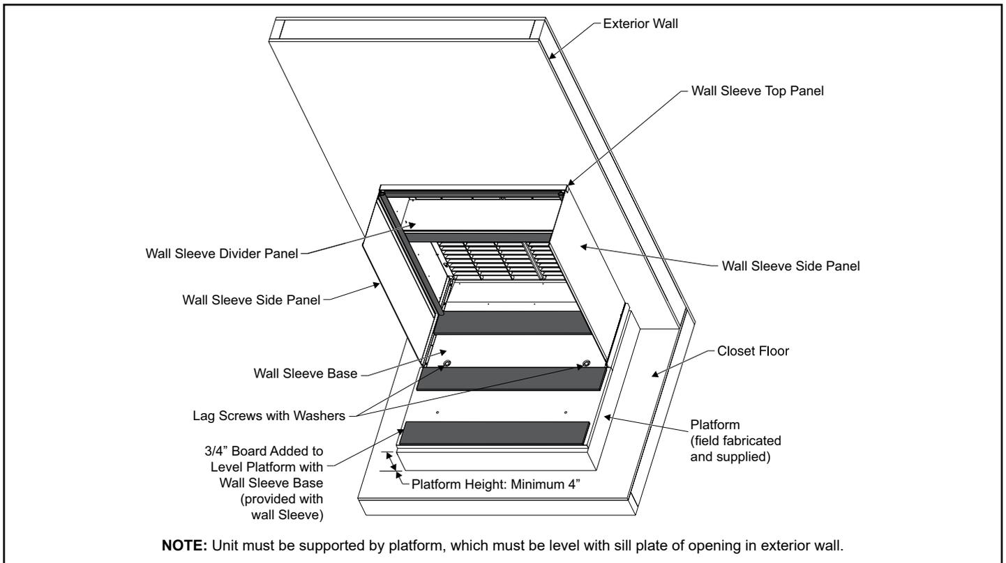
**Figure 3. Wall Sleeve and Louver Kit Installation**
