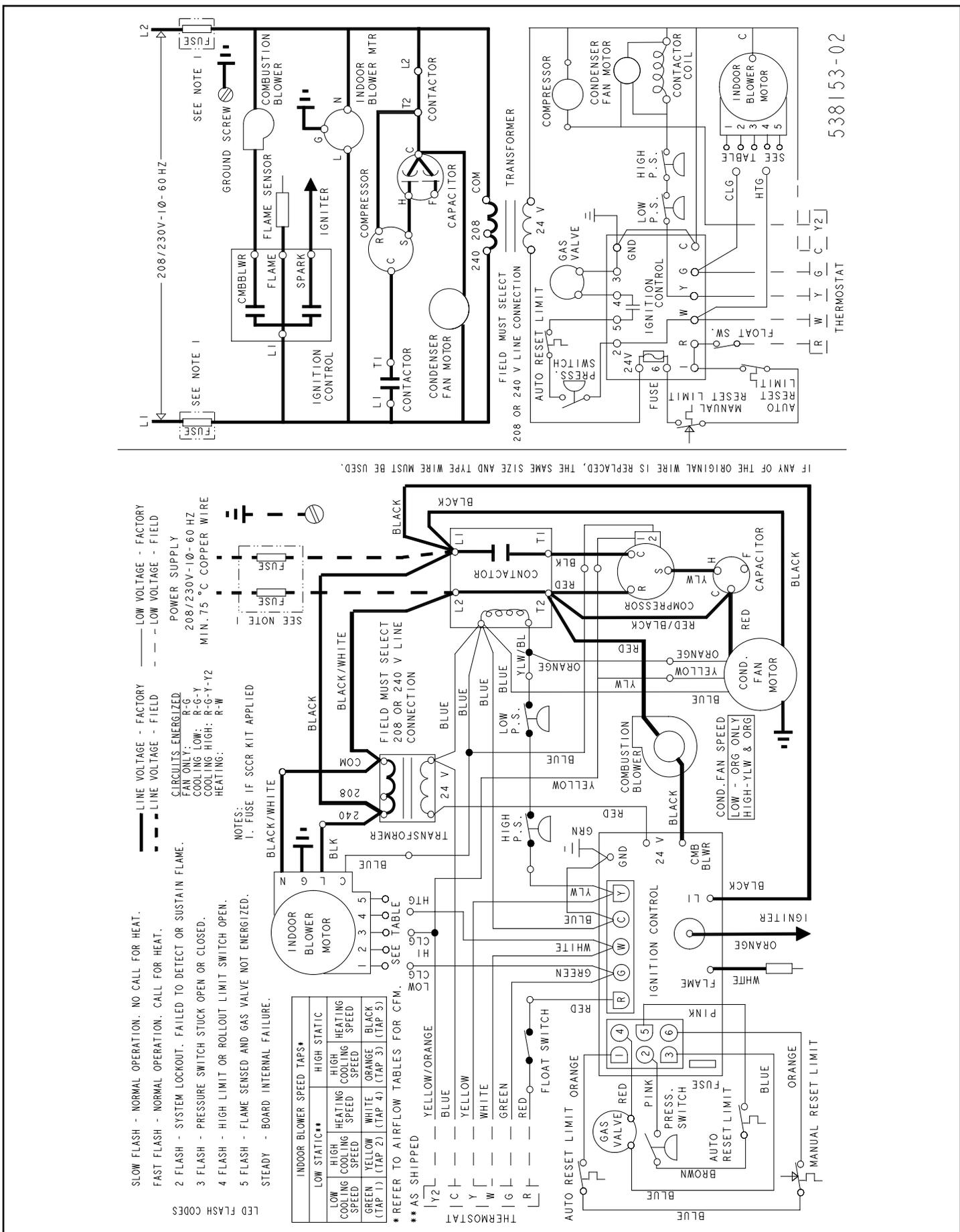
Figure 14. Wiring Diagram - MGE 3 Ton
